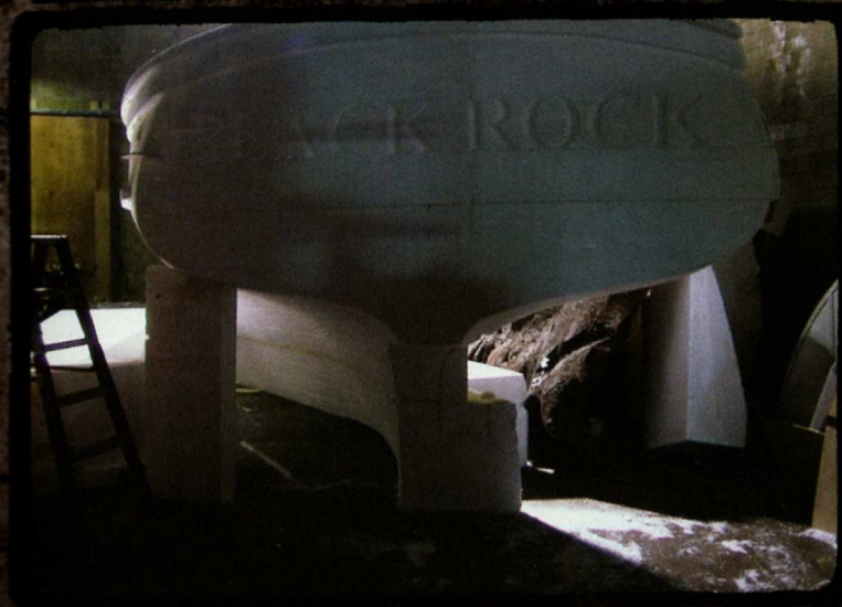
Several blocks of urethane foam are used to sculpt the life-size sections required of the Black Rock
